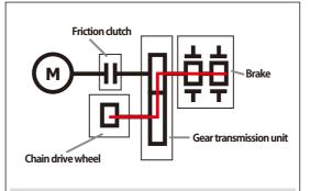
Friction clutch is not in the load path when chain hoist is disconnected from power supply.
